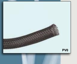
Protect-Fast™ TELCOM Braided Sleeving is an efficient solution allowing for easy installation of wires or bundles of cable. It is a tough, lightweight method used to contain and protect cable assemblies, hoses and wire harnesses from abrasion and cutting.
