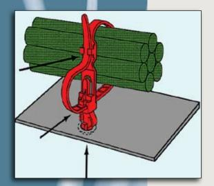
The Pull-Mount cable tie installs from the bottom of the panel. The high strength button head snaps fast and easily into a 3/8" (9.5 mm) diameter hole inside a panel with a thickness range from 0.045" (1.1 mm) to 0.100" (2.5 mm). The cable tie loops around the cables to secure the bundle. The excess cable tie is pushed through the releasable latch mechanism and the retaining tabs to create a secure fit, eliminating the need to cut off excess.
